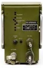
4 – This was the last packet radio made for ARPA. The so-called low cost radio was used in large to test network routing algorithms rather than in the field. The only original field Packet Radio is in the Internet Van outside. Packet Radio was the world's first mobile digital network and basis for internetworking.
