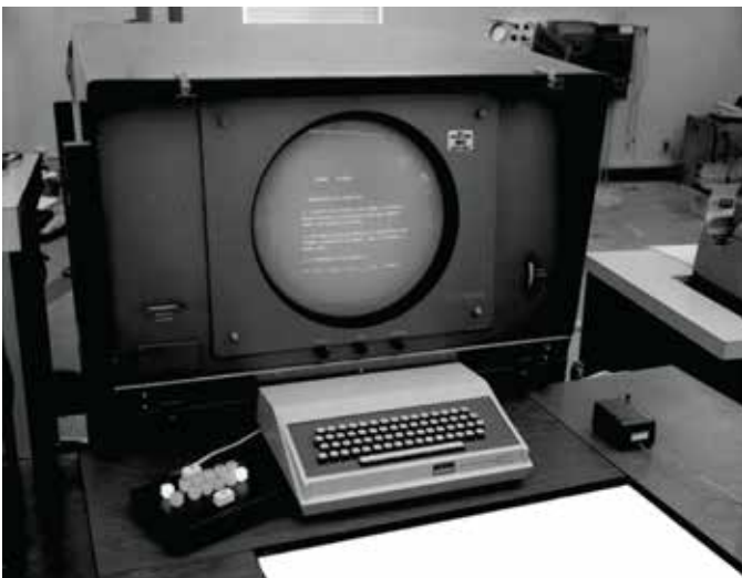
Close-up view of the workstation with its keyboard, command buttons, and mouse.
