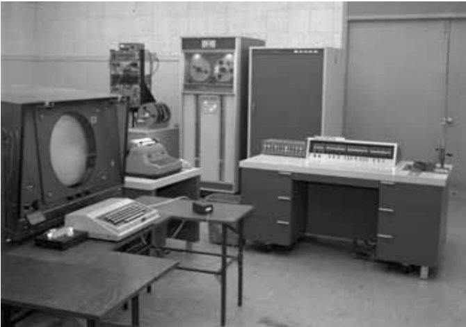
The workstation, with mouse, and the CDC 160A computer to which it was attached.
