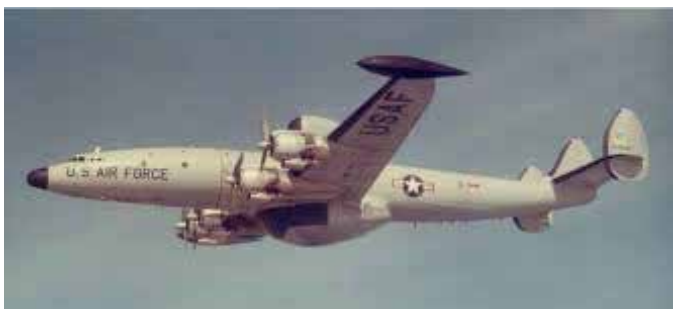
An Air Force Super Constellation configured as an early warning radar plane.
