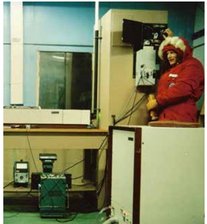
Figure 4. Norm in Antarctica operating a lidar receiver through a homemade 24-in telescope.
